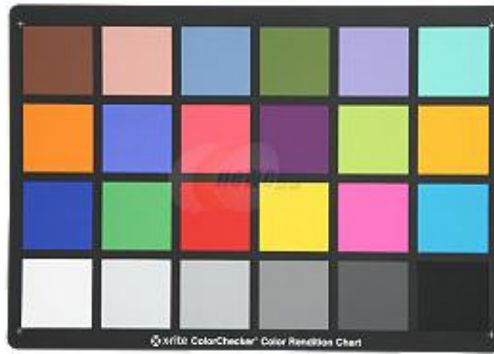
Figure 2-8. X-Rite ColorChecker chart that was used in (Chung et al. 2010) to analyze variations of calibration factor over time for the HDR photography in a daylit interior scene.
