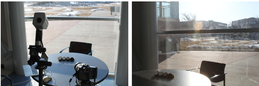
Figure 3-32. Calibration scene with a wider dynamic range for obtaining the RC of camera/lens combination
