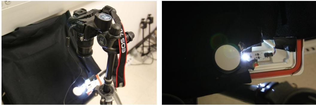
Figure 3-48. Experimental setting for making an HDRI of a single LED chip
