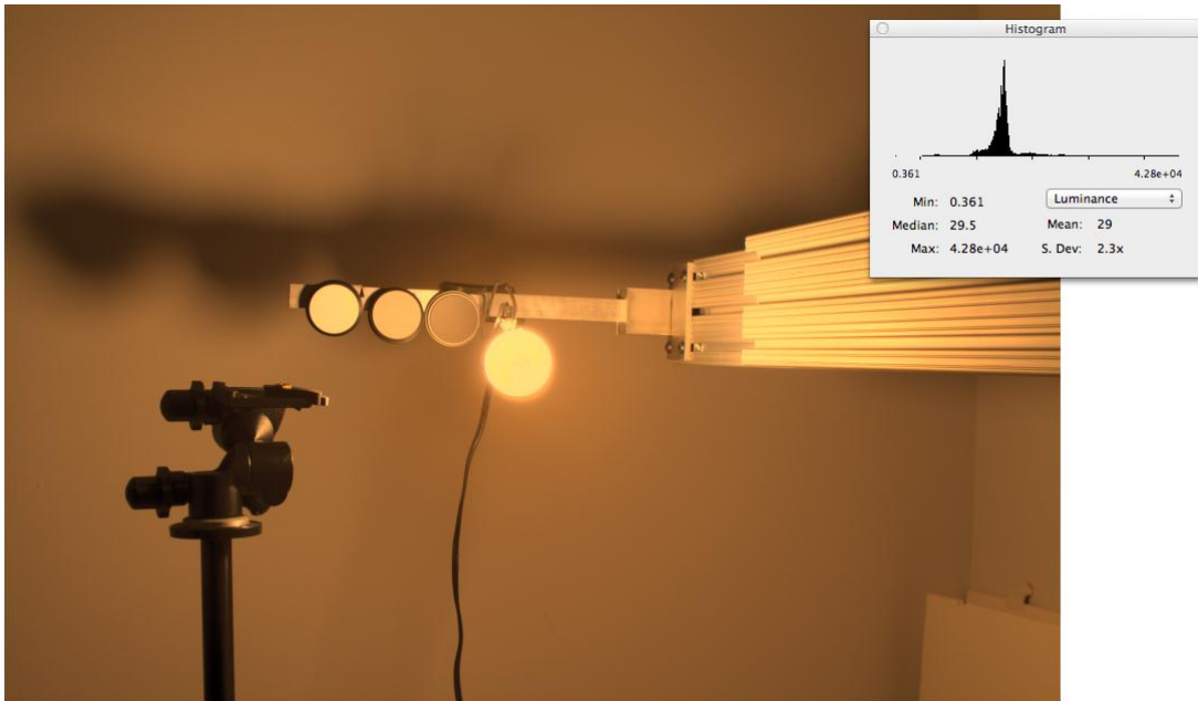
Figure F2. HDRI of incandescent light source captured with CANON EOS 7D fitted with 28-105mm zoom lens at 28 mm
